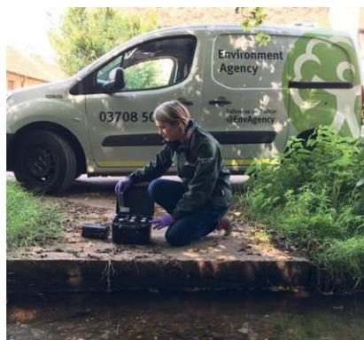
[Figure 1: Environment Agency agent Karen Irwin using a Fluidion ALERT LAB for E.coli field measurements.]
