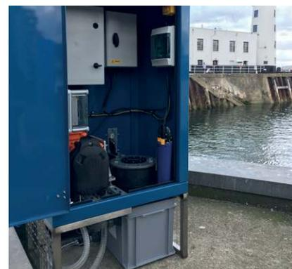
[Figure 2: Environment Agency water quality monitor deployed at Scarborough Harbour. The Fluidion ALERT System is visible at the bottom right.]
